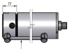
Transfer Tube can be welded or use fittings
