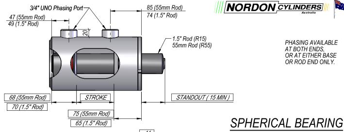
PHASING AVAILABLE AT BOTH ENDS, OR AT EITHER BASE OR ROD END ONLY.
