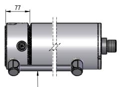
Transfer Tube can be welded or use fittings
