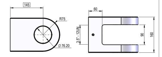
NOTE: ALL THREADS MACHINED TO 2A/B SPECIFICATION. ALL PIN HOLES MACHINED TO D9 TOLERANCE.
