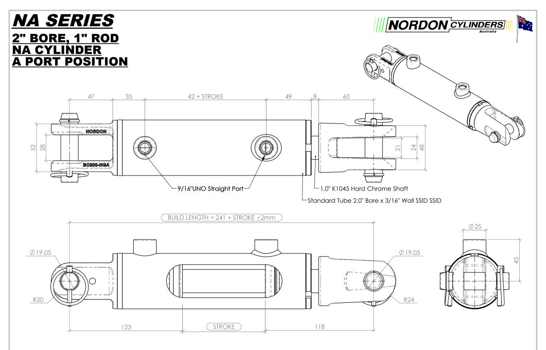
NOTE: ALL THREADS MACHINED TO 2A/B SPECIFICATION.
