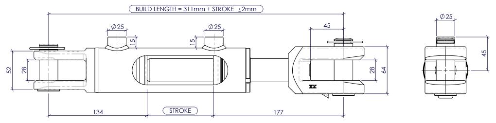
NOTE: ALL THREADS MACHINED TO 2A/B SPECIFICATION.
