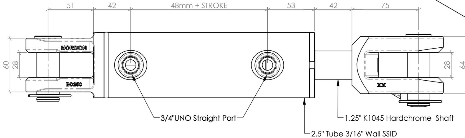
BUILD LENGTH = 311mm + STROKE ± 2mm
