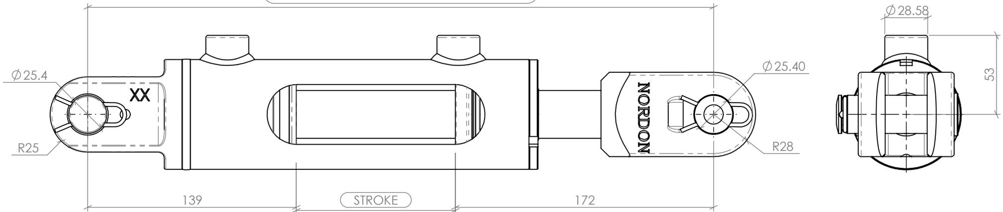
NOTE: ALL THREADS MACHINED TO 2A/B SPECIFICATION.
