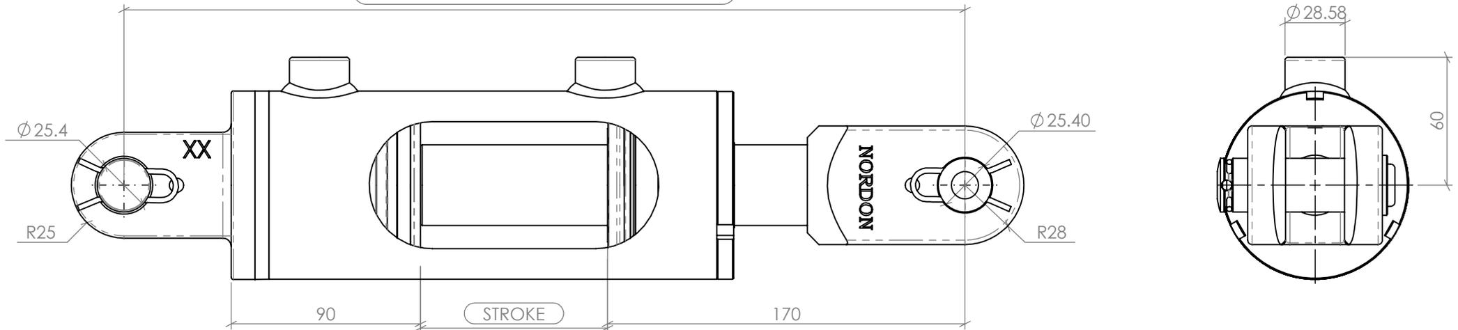
NOTE: ALL THREADS MACHINED TO 2A/B SPECIFICATION.
