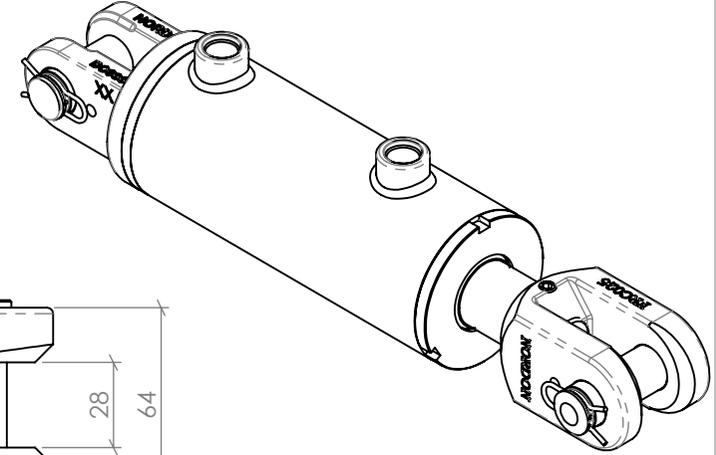
BUILD LENGTH = 311mm + STROKE ± 2mm
