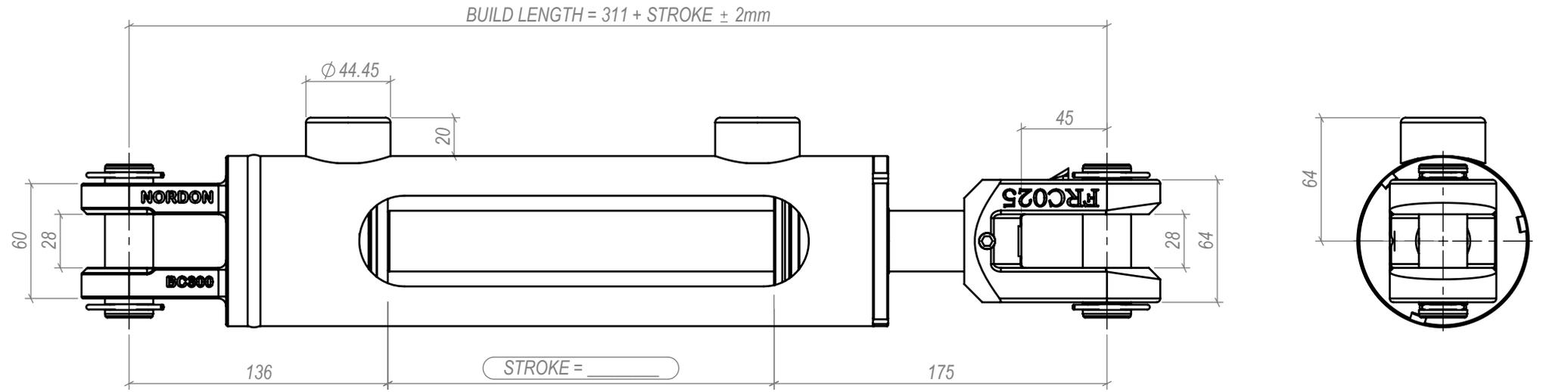
NOTE: ALL THREADS MACHINED TO 2A/B SPECIFICATION.
