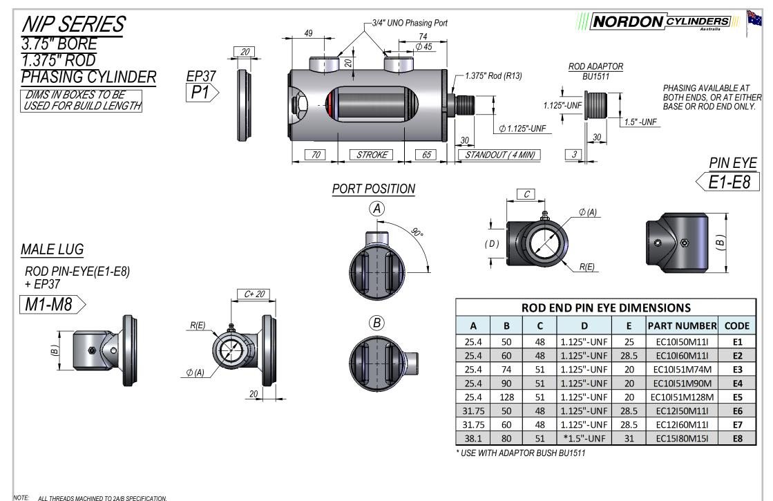
NOTE: ALL THREADS MACHINED TO 2A/B SPECIFICATION. ALL PIN HOLES MACHINED TO D9 TOLERANCE.
